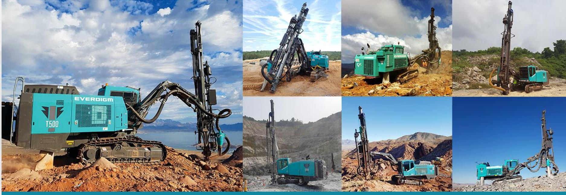
Blast-hole Drill rig
